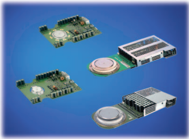
Fig. 3 Standard IGCT sizes
